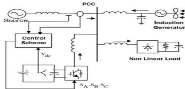
Fig 4.1 STATCOM connected to grid with renewable energy source
