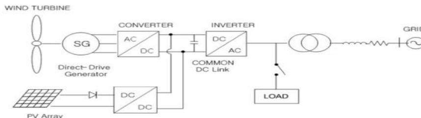
Fig 3.1 wind and PV system connected to grid
