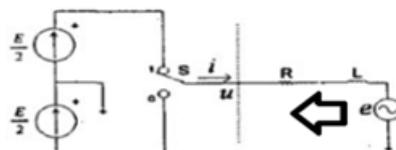
Fig 4.3 Single phase voltage source inverter
