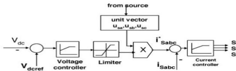
Fig 4.6 Bang-bang current controller
