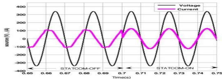
Fig 4.8 Output waveforms of voltage and currents when STATCOM connection and not connected to grid
