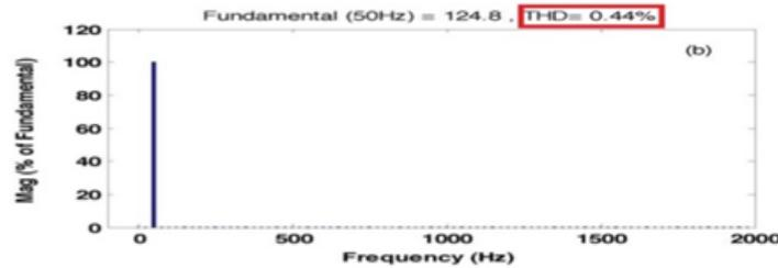
Fig 4.7 THD for Bang-Bang current controller
